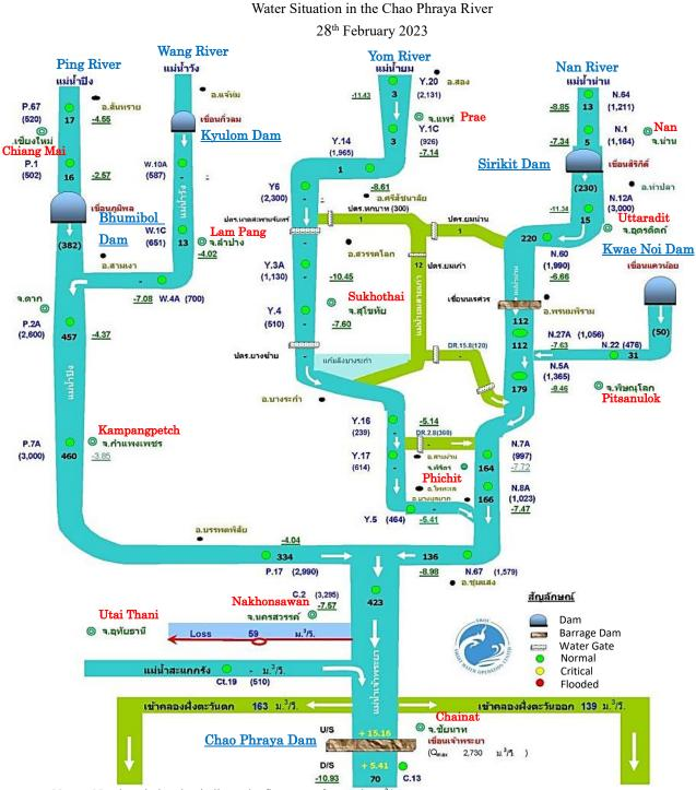
**Note**: - Numbers in bracket indicate the flow rate of water in m<sup>3</sup>/sec.
