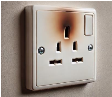
Figure 3: Power outlet burnt
